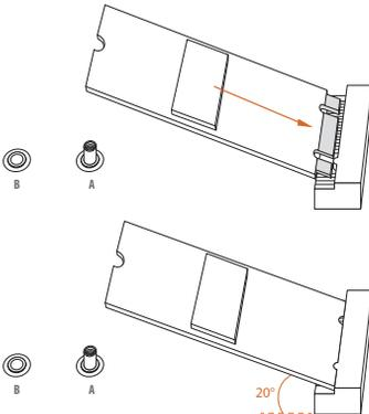
Align and gently insert the M.2 SSD module into the M.2 slot. Please be aware that the M.2 SSD module only fits in one orientation.
