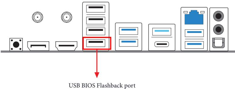
ASRock BIOS Flashback feature allows you to update BIOS without powering on the system, even without CPU.
