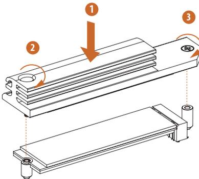
Tighten the screws with a screwdriver to secure the module and M.2 heatsink into place in the order shown. Tighten screw opposite the M.2 connector first (2), and then tighten the one next to the M.2 connector (3).
