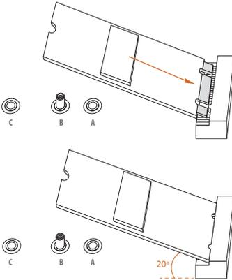
Align and gently insert the M.2 SSD module into the M.2 slot. Please be aware that the M.2 SSD module only fits in one orientation.
