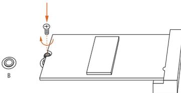
Tighten the screw with a screwdriver to secure the module into place. Please do not overtighten the screw as this might damage the module.
