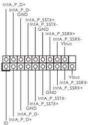
Front Panel Type C USB 3.2 Gen2x2 Header
